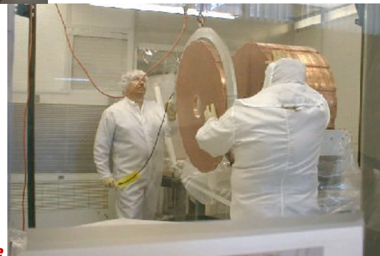
FCal1 copper matrix stacking
