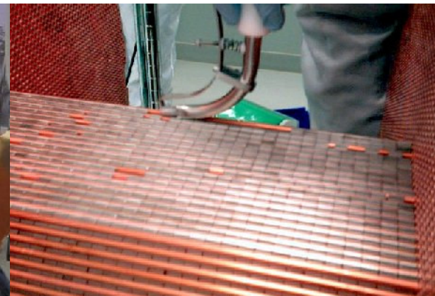
FCal2 and 3 assembly; insertion of tungsten slugs
