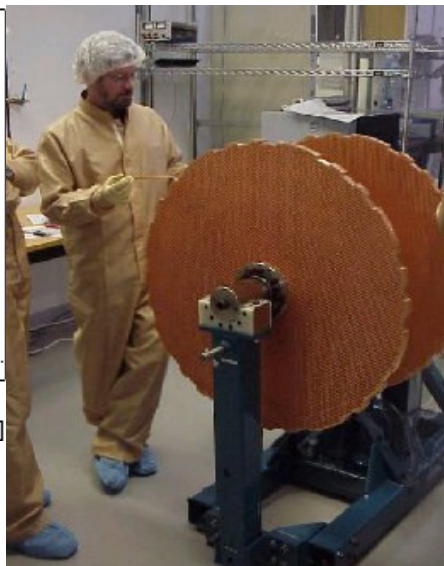
FCal2 and 3 assembly; insertion of tungsten slugs
